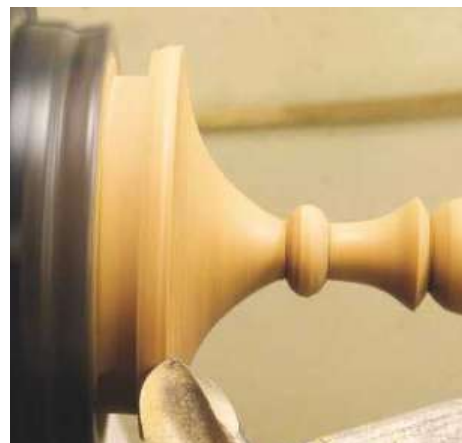
▲ Pic.30 Les likes to put this detail on all his bases, undercutting the edge of the base to create a shadow. Give yourself enough clearance from the chuck to be able to make this cut
